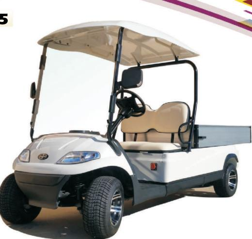
**ITALCAR INDUSTRIAL SRL** | Via Bruino, 36 | 10040 Rivalta di Torino (TO) Tel. +39 011 9040225 | Fax +39 011 9032986 | info@italcar.com | www.italcar.com 48 volt with AC system 8 x 6v lead-acid batteries 205/50-10 aluminum rims front & rear lights hydraulic brakes on 4 wheels + handbrake
